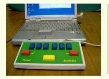
**BrailleKey** provides either Universal computer Braille or UK computer Braille as ASCII characters into any application as well as being a direct interface to Braille devices such as printers.
